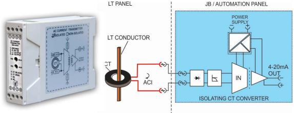
YUTECH's Precision CT Converters Sense the CT Load and Convert the Signal to Isolated 4-20mA Signal which is given to PID Controller which gives a very finely tuned Output to the CSD Valve thus linearly controlling the Massecuite Intake to Centrifuge.
